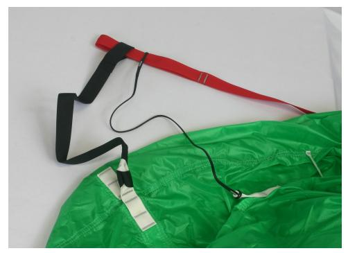
Multi-2 Bridle Attachment: Connect the Multi-2 components to your canopy using a larks head knot.
