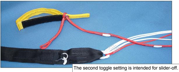
The second toggle setting is intended for slider-off. The shorter toggle position allows for a more responsive turn and flare.
